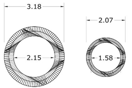
Figure 4. Porta and IVC cuffs front view. Calipers suitable for rats weighing 180-270 g are represented.
