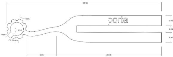
Figure 1. Porta handle stencil. If printed with a scale 1:1 can be used to guide the handle shaping. Click here to view larger figure.
