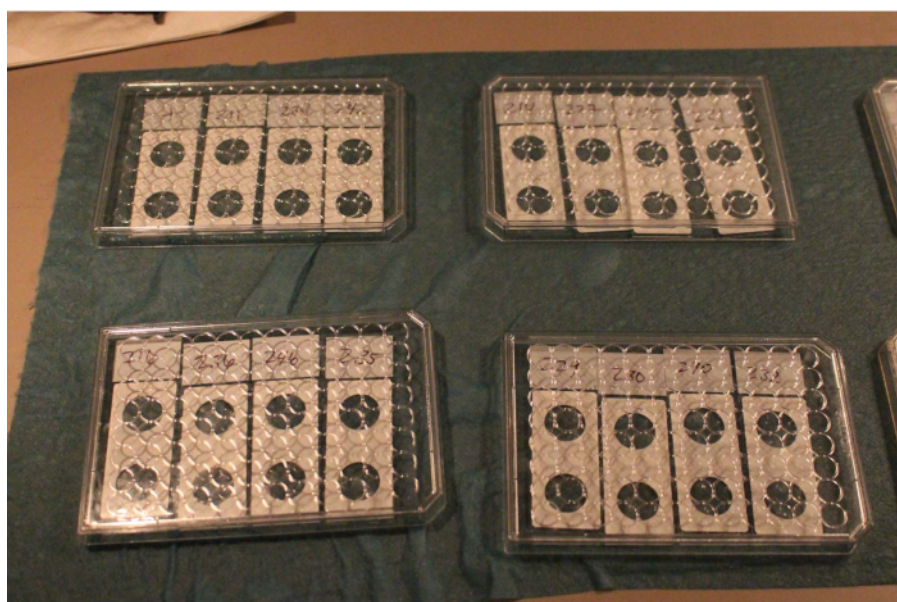
Figure 2: Simple humidity chamber created with a wet paper towel and cell culture plates. A simple humidity chamber using a wet paper towel and cell culture plates allows for field-based application. Please click here to view a larger version of this figure.
