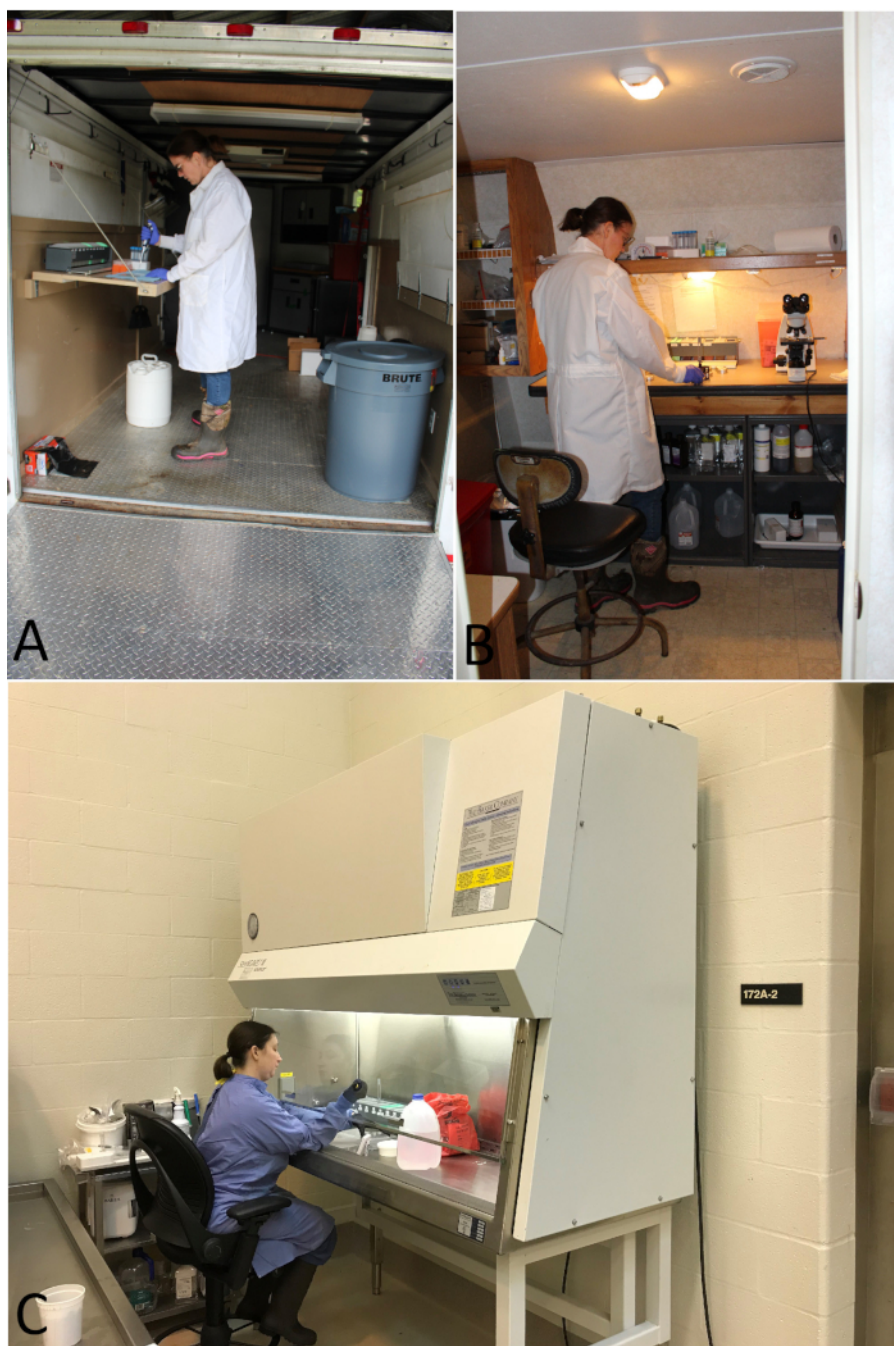
Figure 5: Representative photographs of DRIT testing facilities used by USDA WS. (A) Mobile testing facility in an enclosed trailer for transport. (B) Recreational vehicle retrofitted for DRIT testing. (C) DRIT testing facility in conjunction with university laboratory. Please click here to view a larger version of this figure.
