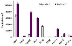
Figure 5: Bacterial binding quantified by cell counts from SEM images. Comparison of cells attached per unit area of surfaces coated with the best 'hit' polymers. Agarose was used as a control 'non-binding' surface, with glass as a control binding surface. Error bars represent standard deviation.
