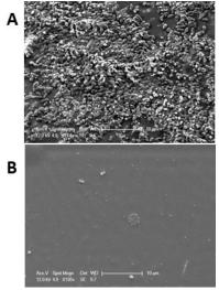
Figure 7: Comparison of bacterial binding on coated and uncoated catheter slices. SEM images show comparison of untreated catheter (cath-1) (**A**) and catheter coated with PA13 (**B**) after incubation with a bacterial cocktail consisting of BacMix-2. Scale bars = 10 μm. Adapted from reference<sup>6</sup>.
