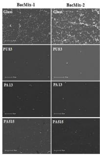
Figure 4: Scale-up experiments with glass cover slips. SEM images showing bacterial attachment on uncoated glass and glass coated with 'hit' polymers (examples chosen from **Table 1**). Scale bars = 20 μm.
