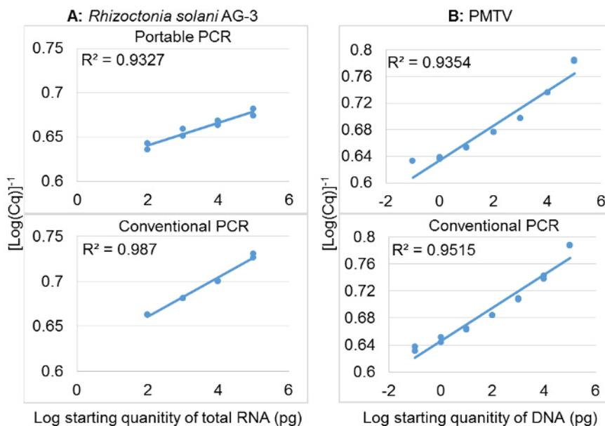
**Figure 5. Detection of other potato pathogens, *R. solani* and PMTV.** Real-time PCRs were performed using the portable thermocycler and the conventional thermocycler. *R. solani* AG3 was detected in total DNA extracted from pure culture using RsTq primers and the RQP1 probe (A) PMTV was detected in total RNA extracted from a PMTV-infected tuber sample using the PMTV-D primer/probe set (B). [Please click here to view a larger version of this figure.](#)
