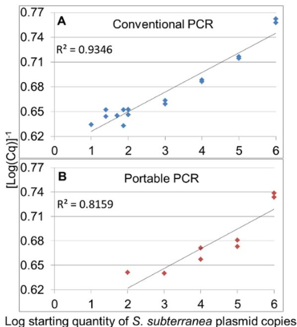
**Figure 2. Comparison of sensitivity between a portable PCR and a conventional lab-based PCR.** Quantification of the pathogen DNA was performed using different amounts of the *S. subterranea* ITS gene ( $10^6$  to  $10^0$  copies) with the SsTQ primers/probe set. Linear regression between log value of *S. subterranea* plasmid DNA and reciprocal Log value of Cq on the conventional thermocycler (A) and the portable thermocycler (B). [Please click here to view a larger version of this figure.](#)
