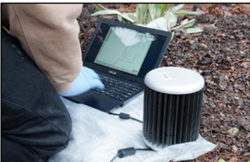
**Figure 1.** Procedure of a portable real-time PCR system for on-site pathogen detection. The protocol is composed of steps in the following order: lysate preparation by brief homogenization (A), magnetic bead-based nucleic acid extraction (B), portable real-time PCR (C), and quantitative data analysis using a laptop computer (D). Note that all steps can be completed on site.
