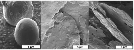
Figure 5: Untreated stainless steel <38 µm (D90) (left), stainless steel powder after attrition milling (middle), and stainless steel powder after PBM milling (right) Please click here to view a larger version of this figure.
