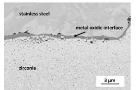
Figure 14: SEM Image of microstructure in the metal-ceramic interface showing the material joint. Please click here to view a larger version of this figure.
