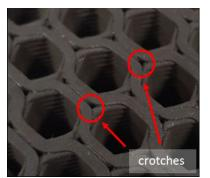
Figure 13: Typical structure of FFF-components resulting from slicing and continuous material deposition. Please click here to view a larger version of this figure.
