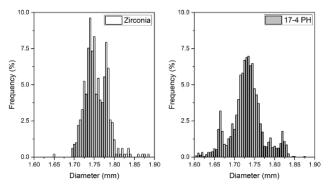
Figure 8: Histograms of the filament diameter for the studied materials. Please click here to view a larger version of this figure.
