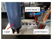
Figure 17: Image of new print head with two FFF-printing heads and one T3DP-printing head (left). Please click here to view a larger version of this figure.
