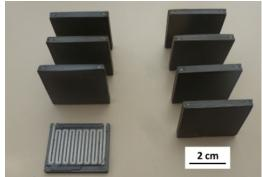
Figure 15: Sintered heating elements made of zirconia and stainless steel Please click here to view a larger version of this figure.
