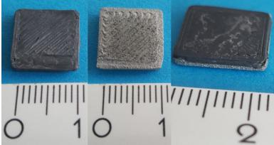
Figure 12: Sintered zirconia sample (left), sintered stainless steel sample (middle), and sintered zirconia-stainless steel-composite (right). All scales in mm. Please click here to view a larger version of this figure.
