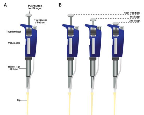
**Figure 6.** Single channel micropipettor. (A) Shown is a sample micropipettor with a plastic tip attached to the bottom of the barrel tip holder. Indicated are the locations of the volumeter, the thumb wheel for changing the volumeter setting, the barrel tip holder, the tip ejector button, and the pushbutton for the plunger. (B) Two-stop plunger system on a micropipettor.
