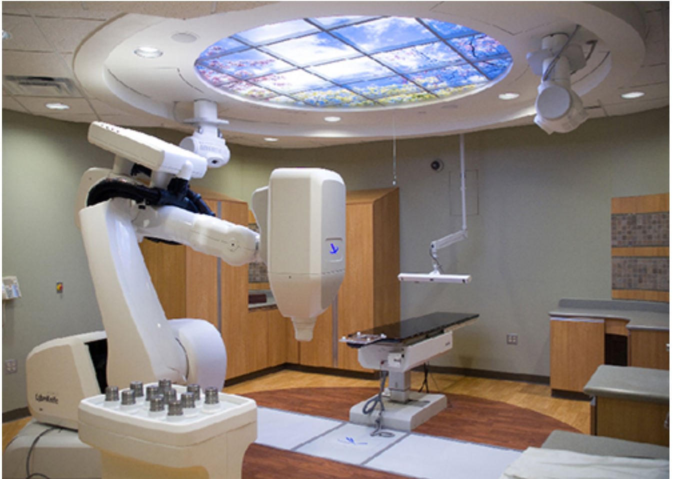
Figure 1. Cyberknife system. A view of the Cyberknife system used for the measurements, with the accelerator head pointing downwards. The water tank can either be placed on the floor, or on the robotic couch visible at the back of the room, depending on the space available above the head.
