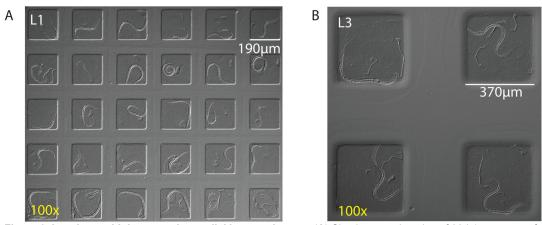
Figure 3. Imaging multiple worms in parallel by zooming out. (A) Simultaneous imaging of 30 L1 worms per frame using 190 x 190  $\mu$ m chambers and a 100X magnification (using a 10X objective) and a 16.6 x 14 mm camera chip. (B) Simultaneous imaging of four L3 worms per frame using 370 x 370  $\mu$ m chambers and 100X magnification and a region of interest of a 16.6 x 14 mm camera chip. Please click here to view a larger version of this figure.
