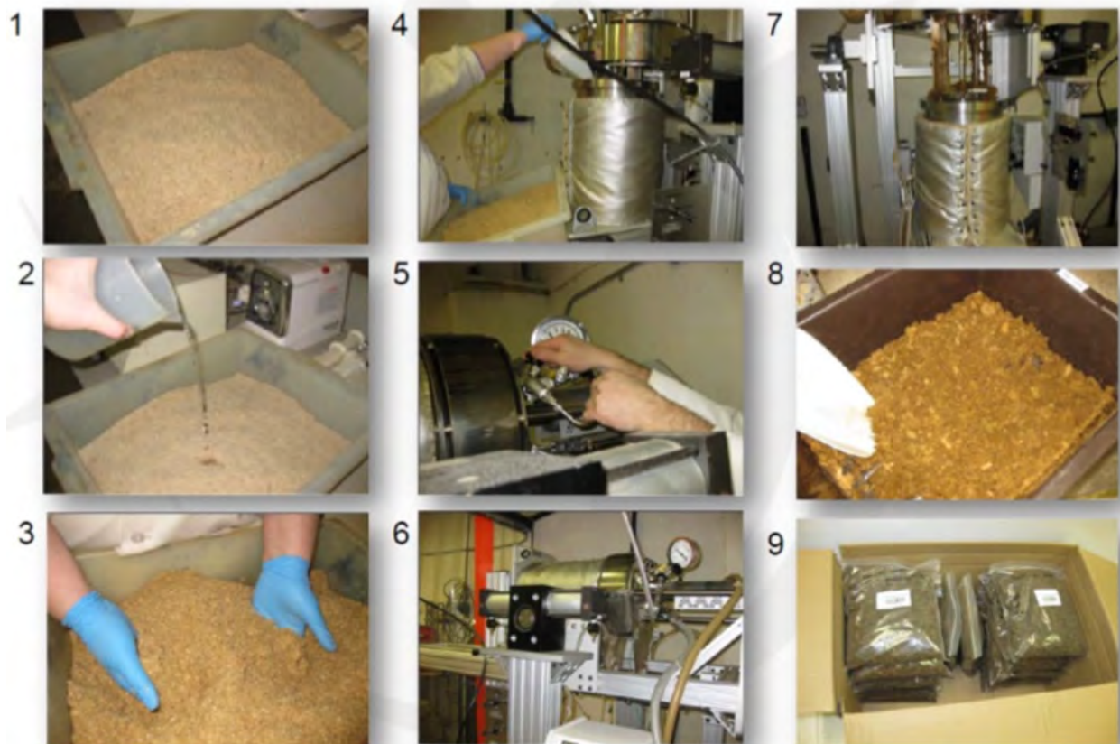
Figure S1. Nine different steps involved in producing AFEX (or Ammonia Fiber Expansion) treated biomass in a lab-scale 5-gallon pressure reactor. 1) Weighing biomass; 2) Adding water; 3) Mixing water with biomass; 4) Loading biomass in the reactor; 5) Applying vacuum and loading ammonia; 6) Running the reaction; 7) Removing the reactor head; 8) Unloading the AFEX-treated biomass; 9) Bagging biomass once dry.
