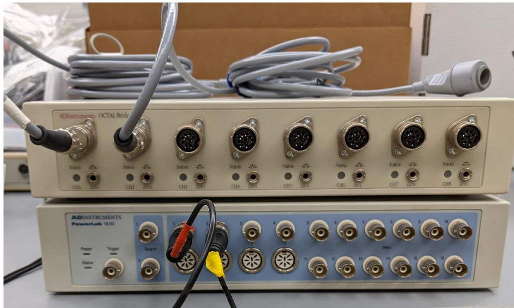
Figure S2: Front panels for ADInstruments PowerLab (bottom) and Bridge Amp (top)
