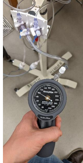
Steps 6-7: Sphygmomanometer for two-point pressure transducer calibration
