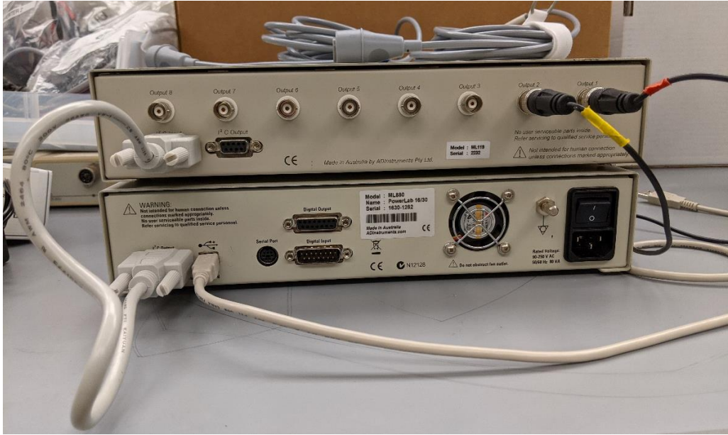
Figure S3: Back panels for ADInstruments PowerLab (bottom) and Bridge Amp (top)
