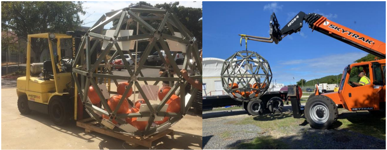
Figure S21: Shell Arks may be attached to a pallet and lifted via a forklift to load them onto vessels or transport them as needed.
