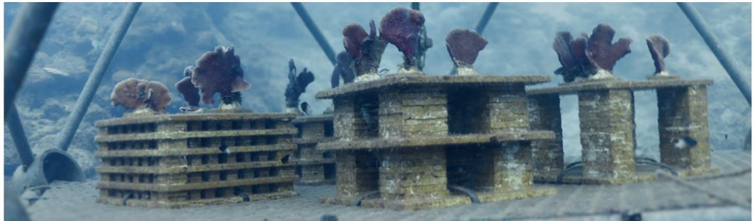
Figure S8: Limestone ARMS can be built with differing internal complexities. Smaller, more numerous internal components yield higher internal surface area, with implications on fouling (biofilms and sessile invertebrate communities) and a correspondingly lower internal surface area to volume ratio. ARMS complexities can be designed based on desired recruitment patterns, with higher complexity ARMS recruiting smaller mobile organisms.
