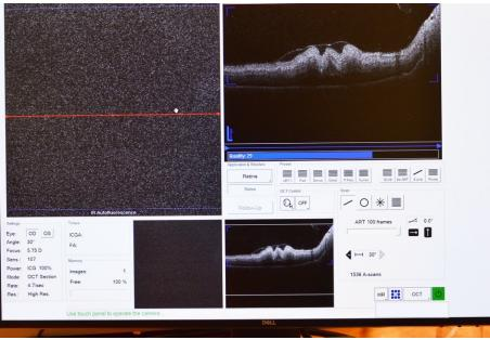
Switch the internal cube back to "R" for IR and Red free imaging for volume acquisition.
