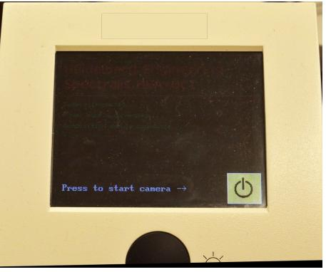
Press section and press IR +OCT. Other default settings are blue. Allow laser to acquire fundus image and OCT image. Rotate black round button to adjust intensity and press the same button to average image 9-100 frames (red arrows).
