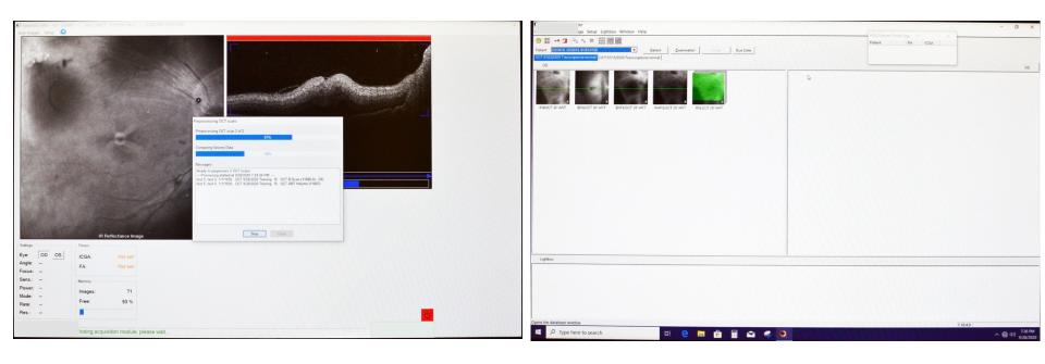
It is recommended to not change the position of the mounting bracket between imaging fellow eyes. If left eye is imaged first, the results will show in the OD Eye column ----->. Right-Click, select all the images, then select 'Exchange OS/OD'. The images will shift to the OS column.
