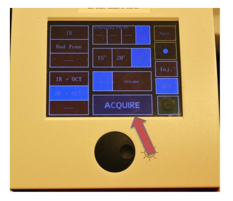
Re-check position so image has not moved or degraded. Press black button for averaging. Press ACQUIRE.
