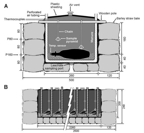
**Figure 1.** Diagrammatic representation of the biosecure compost system comprising straw bale walls and floor, plastic sheeting enclosure, loose straw base, cattle carcasses, manure, perforated plastic ventilation tubing, and air vents, as well as experimental amendments (leachate port, sample retrieval pyramids and temperature sensors. (A) Transverse view (cross section). (B) Longitudinal view (side wall removed). All dimensions are in cm. From Xu et al. (2009)<sup>2</sup>
