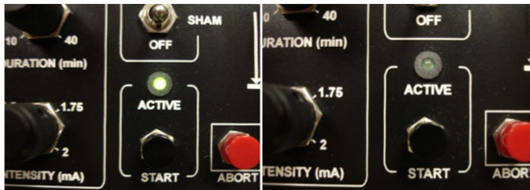
Figure 8. Delivery of active (left) and sham (right) mode by conventional tDCS device. From DaSilva, *et al.*<sup>19</sup>.
