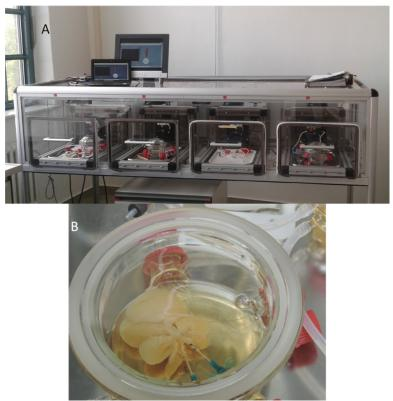
**Figure 1. Bioreactor system. A)** This bioreactor system was custom-made. It maintains the organ models at 37 °C and 5% CO<sub>2</sub>. The flow rates of the peristaltic pumps can be regulated individually. **B)** The liver is placed in a growth chamber and connected to the perfusion circuit, which consists of a peristaltic pump, a medium reservoir, a bubble trap and a pressure sensor. Please click here to view a larger version of this figure.
