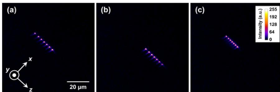
**Figure 9:** Adjustment of the axial potential of the trapped ions in a linear chain. (a) Seven ions at the center of the trap. (b) The ions were shuttled tens of micrometers. (c) The ion string squeezed in the axial direction. This figure is best viewed as a movie, which is separately uploaded. [Please click here to view a larger version of this figure.](#)
