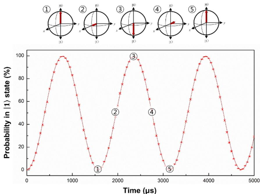
**Figure 10: Experimental results of Rabi oscillations between the  $|0\rangle$  and  $|1\rangle$  states.**  $|0\rangle$  is defined as the  $^2S_{1/2}|F=0, m_F=0\rangle$  state of the  $^{171}\text{Yb}^+$  ion, and  $|1\rangle$  is defined as the  $^2S_{1/2}|F=1, m_F=0\rangle$  state. The Rabi oscillation is induced by a 12.6428-GHz microwave. Bloch spheres above the plot show the corresponding quantum states at different times. [Please click here to view a larger version of this figure.](#)
