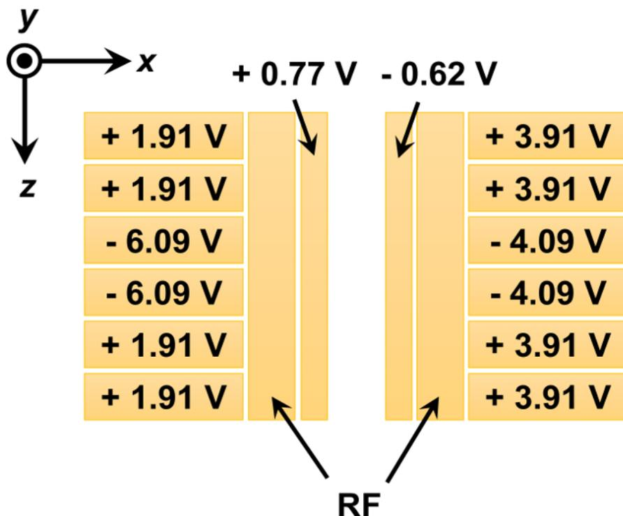
**Figure 4: An example of the DC voltage set used to trap ions.** The voltages applied to the inner rails can compensate for the asymmetric electric field in the horizontal direction to tilt the principal axes of the total potential in the transverse plane. The axial trap frequency generated by the voltage set was 550 kHz. [Please click here to view a larger version of this figure.](#)
