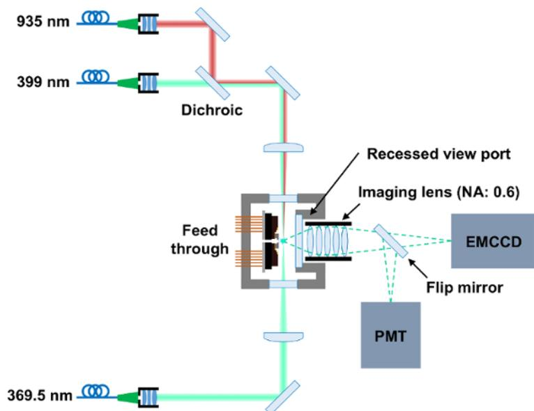
**Figure 5: Schematic of the optical setup.** Three diode lasers are aligned to overlap at the trapping position. The recessed viewport of the UHV chamber allows the imaging lens to be placed as close as possible to the chip surface. A flip-mirror placed between the imaging lens and the EMCCD allows for the selective monitoring of the ion fluorescence using either a photon multiplied tube (PMT) or an EMCCD. [Please click here to view a larger version of this figure.](#)
