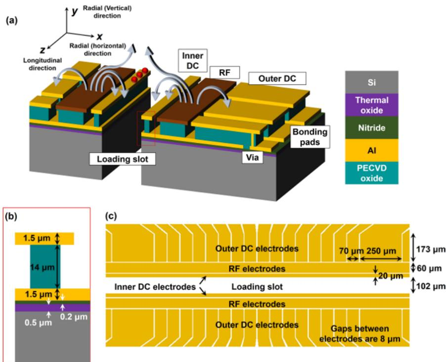
**Figure 1: Schematic of the surface ion trap.** (a) The red dots represent the trapped ions. The brown and yellow electrodes indicate the RF and DC electrodes, respectively. The gray arrows show the direction of the electric field during the positive phase of the RF voltage. Note that the schematic is not drawn to scale. (b) The vertical dimensions of the electrode structure. (c) The lateral dimensions of the electrode structure. [Please click here to view a larger version of this figure.](#)
