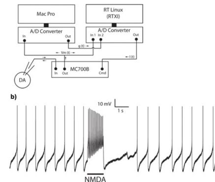
**Figure 1:** Application of a NMDA receptor conductance using the dynamic clamp technique. A. Hardware setup illustrating the connections between the intracellular recording rig and dynamic clamp computer. B. A burst of action potentials is evoked by application of a 40nS NMDA receptor conductance in a whole cell recording from a substantia nigra pars compacta dopaminergic neuron.
