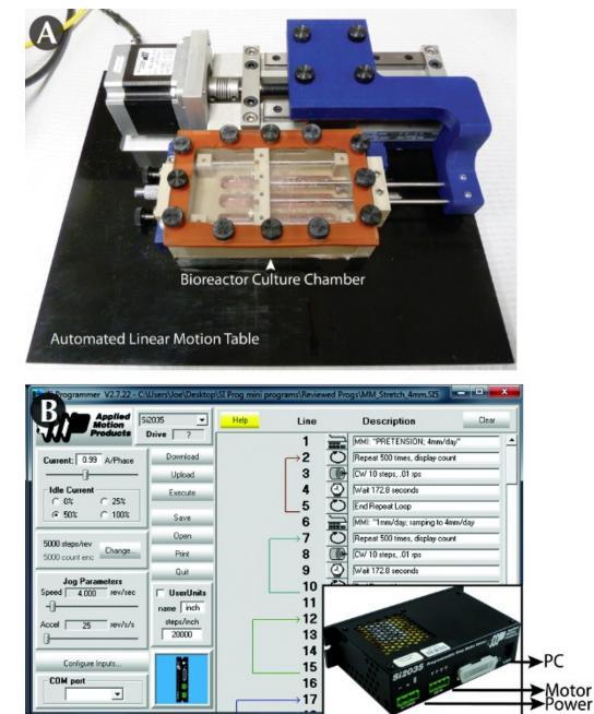
Figure 1. Axon Stretch Growth Bioreactor System. (A) Bioreactor culture chamber & Automated linear motion table, (B) Step motor drive controller and Si Programming software.
