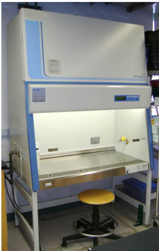
**Figure 10.** Laminar flow hood used to prevent contamination of solutions and cultures. Shown is a biosafety cabinet approved for work with BSL-2 organisms.
