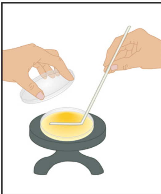
Figure 5. Spread-plate technique with a turntable and glass spreader. After the agar plate is placed on a turntable, a small volume of sample (0.1 to 0.2 ml) is dispensed aseptically onto the center of the plate using a micropipettor. The spreader is sterilized by dipping it into a beaker of ethanol then passing it through the flame of the Bunsen burner to ignite excess ethanol. Before making contact with the sample, the spreader should be cooled by touching it to the agar near the rim of the plate. The spreader is gently moved back and forth through the sample across the plate while the turntable is slowly spinning. This action allows gradual but even spreading of the sample across the agar surface. After closing the lid, the plate should be set on the bench top undisturbed for at least 5 minutes to allow the sample to absorb completely into the agar prior to inverting the plate for incubation.
