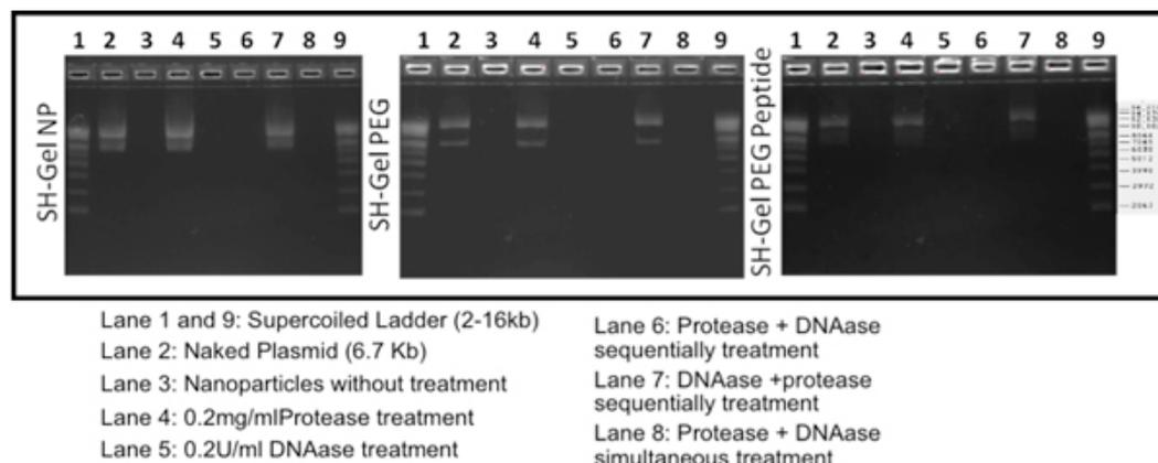
**Figure 2.** Stability of plasmid DNA encapsulated in thiolated gelatin, PEG-modified thiolated gelatin, and EGFR peptide-modified thiolated gelatin nanoparticles by agarose gel electrophoresis. The nanoparticles were treated with 0.2 mg/ml of protease to prove plasmid DNA encapsulation within the nanoparticle matrix
