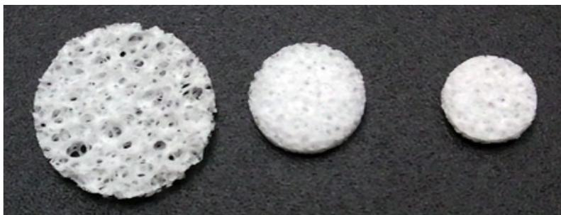
**Figure 1.** Dehydrated PVA sponge disks in three different sizes.
