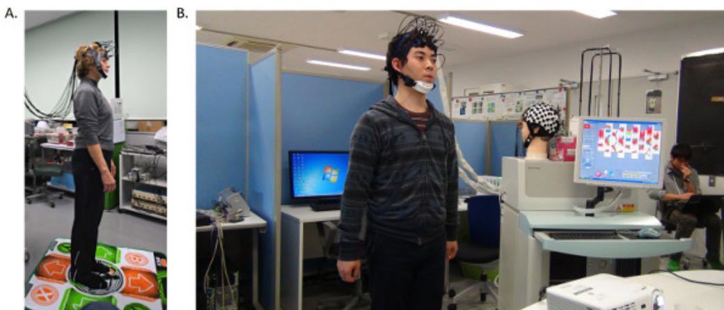
Figure 7: fNIRS data collection during dance game play. (A) Subjects stand to play the game using the block paradigm on a standard dance game mat while being tethered to the NIRS machine. (B) Alternative view of data collection showing raw data on background screen collected in real time from subject. Please click here to view a larger version of this figure.
