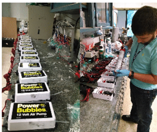
Figure 1. Sealing and preparing recirculation pumps. Sealing recirculation pumps for field deployment.
