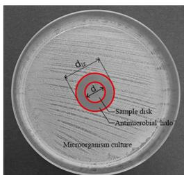
**Figure 1: Measurements for the normalized width of the antimicrobial "halo".** This panel shows the diameter of the inhibition zone ( $d_{iz}$ ) and the disk diameter ( $d$ ). [Please click here to view a larger version of this figure.](#)
